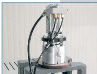
CODE 40097: Sgancio utensile ISO 40 pneumatico ISO 40 Spindle shaft with hydraulic lock and release system
